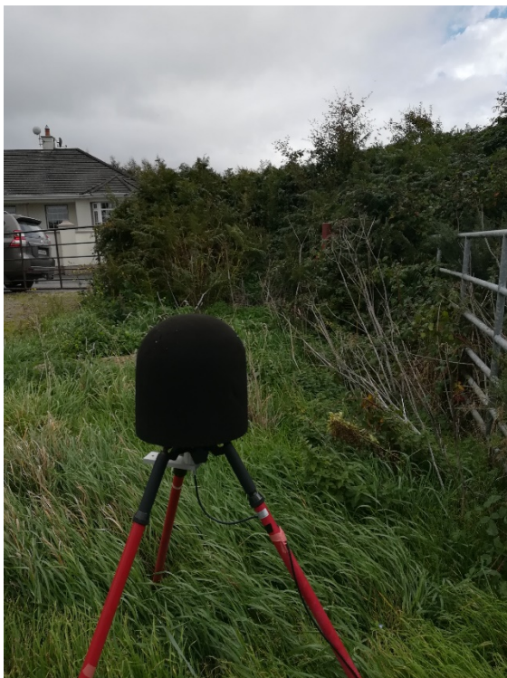
Location N2: Noise monitor in-situ
