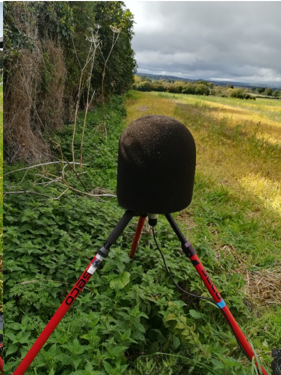
Location N1: Noise monitor in-situ
