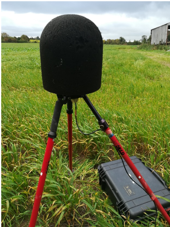
Location N3: Noise monitor in-situ
